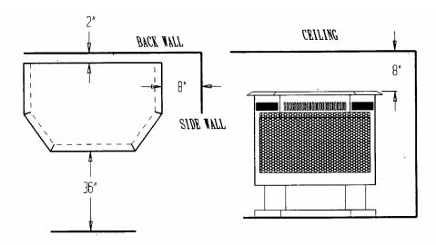
THIS APPLIANCE SHALL BE INSTALLED ON A METAL OR WOOD PANEL THAT EXTENDS THE FULL WIDTH AND DEPTH OF THE APPLIANCE WHEN INSTALLED ON A COMBUSTIBLE SURFACE OTHER THAN WOOD.
